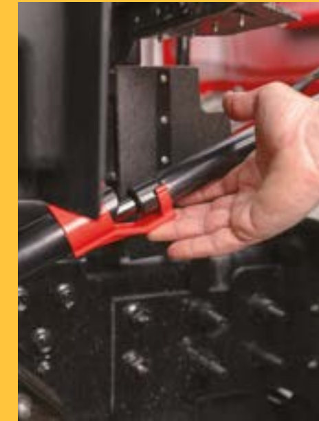
Integrated hood safety latch helps prevent the hood from blowing down on windy days.
