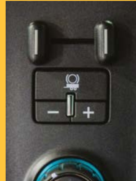
The Trailer Brake Controller helps drivers maintain control while towing.
